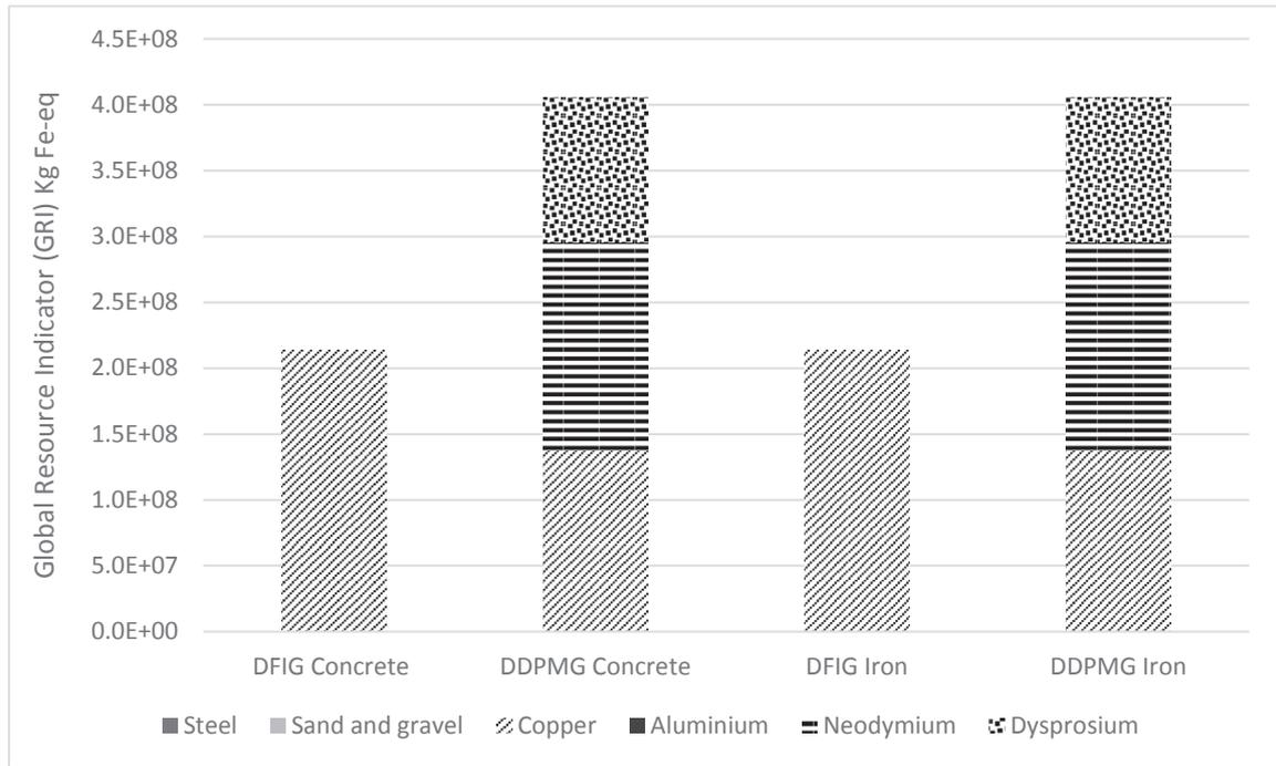
**Fig. 5.** GRI results for the 4 wind turbines technologies at short term.
