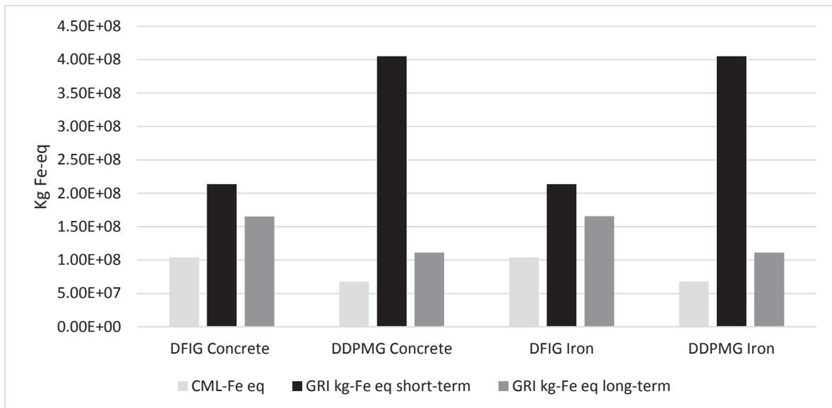
**Fig. 6.** Comparison between four different types of wind turbines (i) CML baseline (ii) short term GRI and (iii) long term GRI in Fe-eq.
